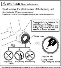
\*If you use a high pressure washer, water will get into the sealed bearings and will rust your bearings. \*If you use a degreaser, it will dissolve the grease out of the bearings.
