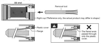
2 Make sure that the flared ends engaged the flange, and then use a hammer to strike the tool head and taking out the right cup.
