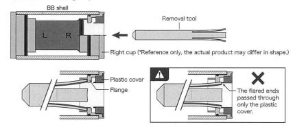
② Make sure that the flared ends engaged the flange, and then use a hammer to strike the tool head and taking out the right cup.
