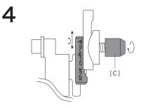
Adjust FD height and angle in accordance with FD technical instructions and tighten the nut [C] to secure the FD assembly.
