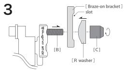
Attach the FD assembly to [Braze-on bracket] on the frame by inserting the bolt [B] through the slot of the bracket, slip [R washer] over the bolt [B], and then install the nut [C] on it.
