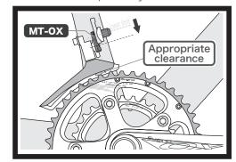
\*Please note that it cannot be used on some frames as FD will interfere with chainstay when it is lowered.
