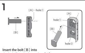
the hole in the base plate [A].
