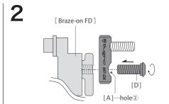
Attach the base plate [A] and [Braze-on styel FD] by inserting the bolt [D] through [A]—hole② into the threads on the FD. Tighten securely.
