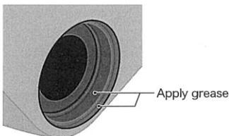
\*If the gasket-ring is damaged or worn, replace it with a new one.
