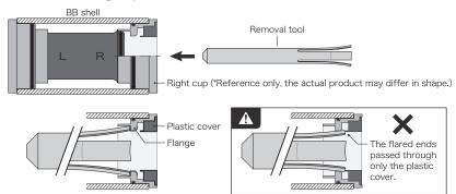
2) Make sure that the flared ends engaged the flange, and then use a hammer to strike the tool head and taking out the right cup.
