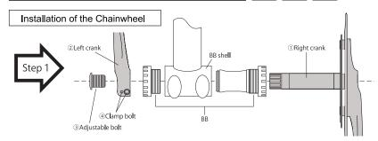
Install the BB to the BB shell according to user's manual of the BB.
