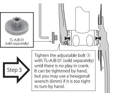
If the crank doesn't rotate smoothly, loosen the
